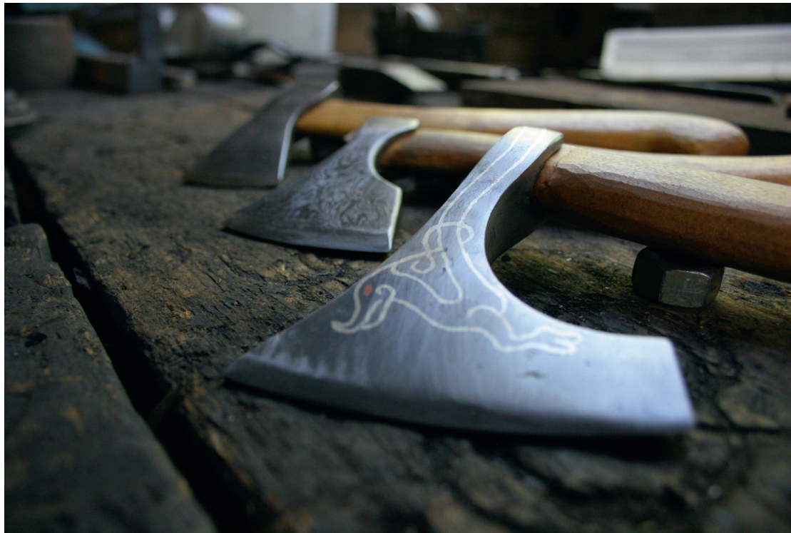
Figure 8: Small camping axes forged by me (2002). One is silver/copper encrusted, the other two are pattern welded. Photography by Gustav Thane.
