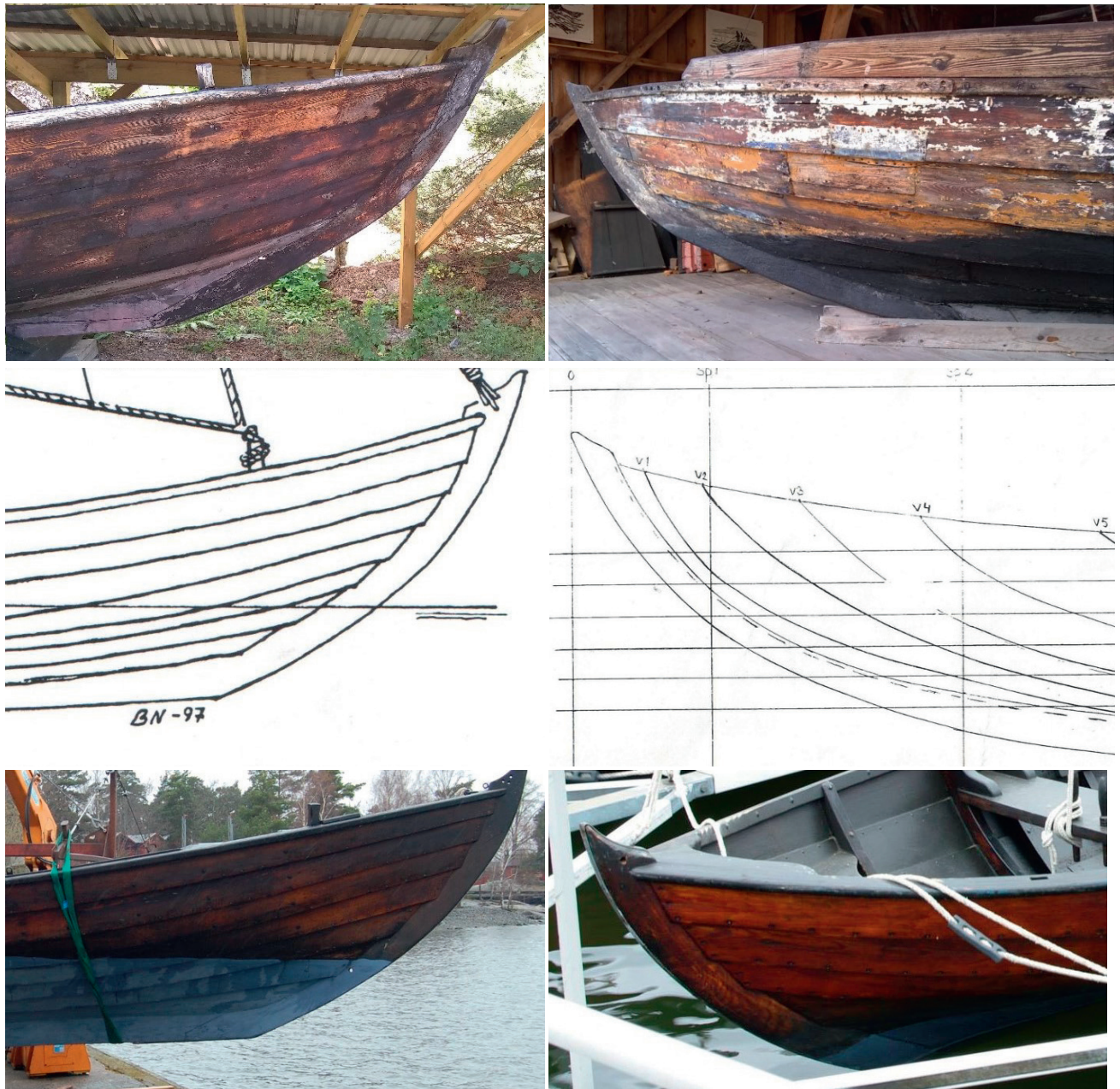
Figure 5 A–F: Two nineteenth-century boats from the Stockholm archipelago, interpreted in reconstructions, but lacking the characteristic shape of the stem. A–B show the original boats, C–D show the line plans from the documents. E–F show the replicas. Images by Fredrik Leijonhufvud.
