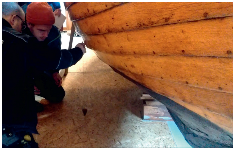
Figure 2: Documentation of a boat using traditional methods which use a plumb line and a tape measure. Photograph by Fredrik Leijonhufvud.
