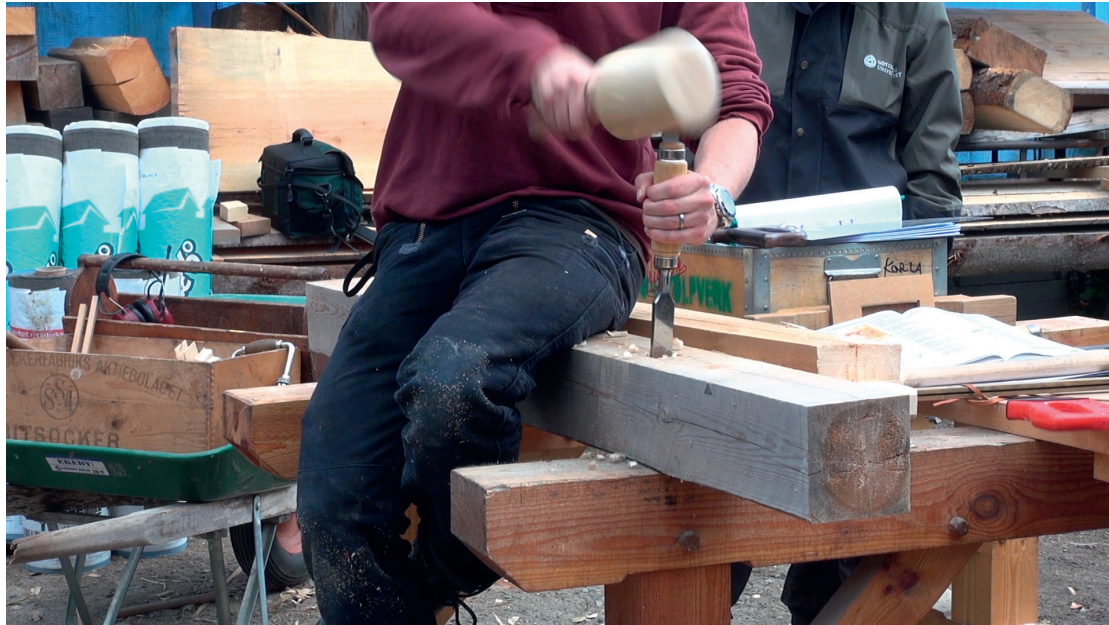
Figure 6: Video sequence of me teaching, demonstrating how I cut a mortice. Click the image to see the video if reading a pdf version, scan the code to the right or go to: https://youtu.be/cBSERnzhn2Y . Video by Ulrik Hjort Lassen.
